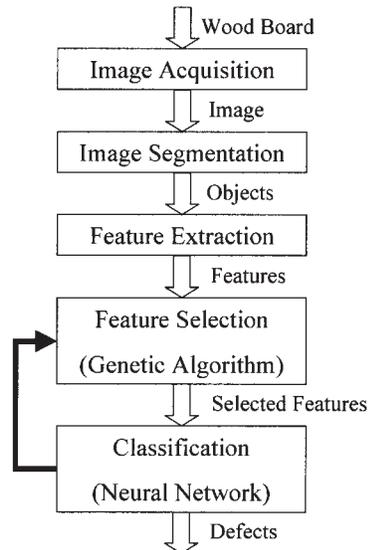
Figure 1. — Automated visual inspection system for wood boards. A feature selection stage based on a genetic algorithm is added to the conventional framework to select an appropriate feature subset as inputs to a neural network classifier.
