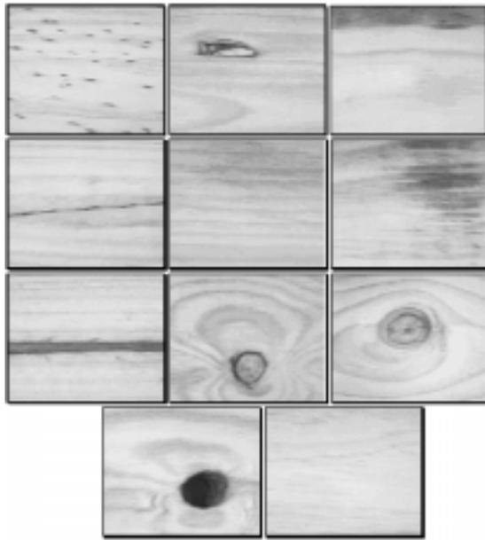
Figure 2. — Image samples of each of the 11 categories considered. In the top row, left to right, birds eye, pocket, and wane; in the second row, left to right, split, blue stain, and stain; in the third row, left to right, pith, dead knot, and live knot; in the bottom row, left to right, hole and clear wood.
