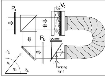
**FIGURE 1.** Experimental setup. Two confocal lenses, (not displayed in the scheme), provide a 1 : 1 image-forming system from the front side of the LCLV to its rear side. The optical feedback loop is closed by a fiber bundle, which is aligned in order to avoid any rotation or shift.  $P_{in}$  and  $P_{fb}$  are, respectively, the input and feedback polarizer. Their orientation with respect to the liquid crystal director is indicated in the left bottom of the figure.
