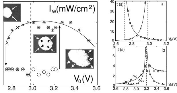
**FIGURE 3.** Bistability and front propagation. On the left,  $I_w$  vs  $V_0$  plot; circles: dark state with writing light off; stars: white state with writing light off; cross: white state with writing light on. On the right, a)  $\tau_r$  (circles) and  $\tau_f$  (cross); b)  $\tau_{on}$  (cross) and  $\tau_{off}$  (circles) as a function of  $V_0$ .
