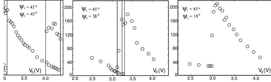
**FIGURE 2.**  $I_w$  as a function of the r.m.s. values of the applied voltage  $V_0$ , for different angles,  $\psi_1$  and  $\psi_2$ , between the polarizers and the liquid crystal director.
