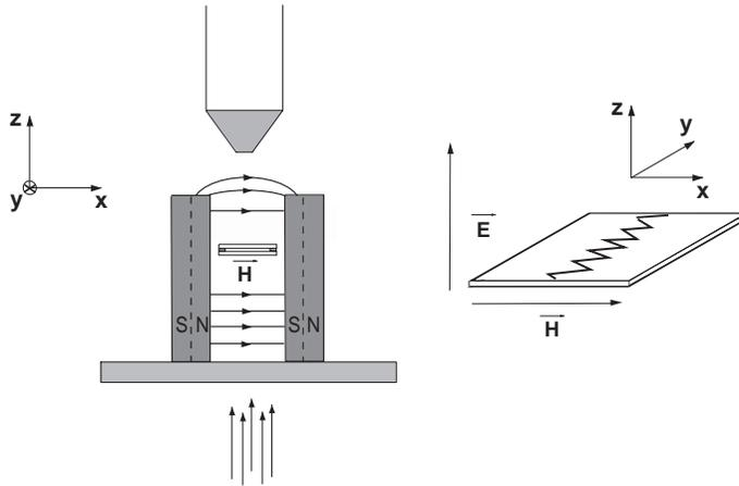
Fig. 1 – Experimental set-up: the sample of liquid crystal is placed between two permanent magnets which determine the homogeneous magnetic field  $\vec{H}$ . The physical phenomena are observed through a polarizing microscope.
