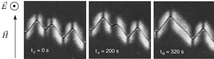
Fig. 2 – Spinodal decomposition of the interface observed through a microscope with crossed polarizers. Due to the orientation of the polarizers, parallel and perpendicular to the magnetic field, the sample looks white as soon as the molecules get partially out of the magnetic plane ( $xz$ ).
