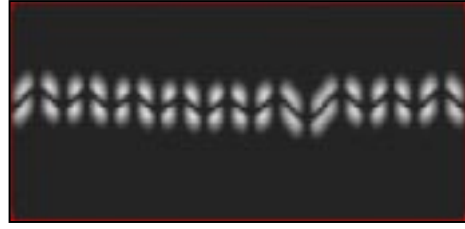
Fig. 6. Numerical simulation of the equation (7) for a high anisotropy of elasticity: K_2/K_1 = 0.056 , K_3 = 1 , \varepsilon = 1 , b = 1 , a = 1 . The picture shows the Y -component of the director in the system.
