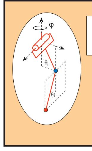
Mechanical analog of a laser close to the 1:1 resonance
