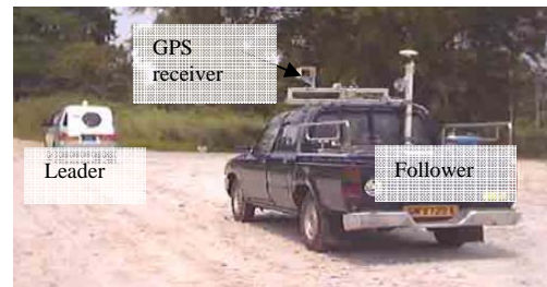
Figure 10. Experimental setup for vehicle following in sub-urban
