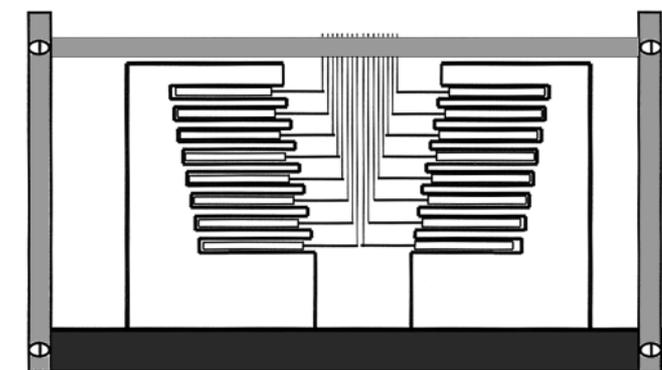
Fig. 2 Schematic diagram showing array of 16 piezoelectric vibrators mounted horizontally in cantilever manner with vertical contactor to touch skin
