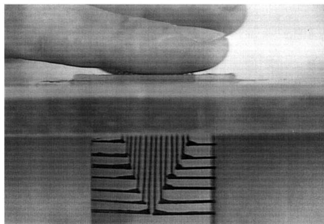
Fig. 4 Array of 16 piezoelectric vibrators and how contactors touch index finger. Acrylic rectangle on top contains 16 circular holes to guide contactors, maintaining 1 mm distance between neighbours
