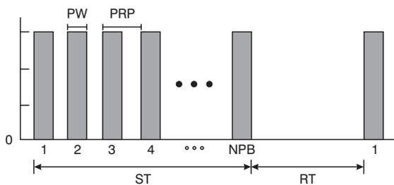
**Fig. 1** Driving waveform composed of burst of rectangular pulses followed by recovery time. Parameters of waveform are pulse width (*PW*), pulse repetition period (*PRP*), number of pulses per burst (*NPB*), stimulatory period (*ST*) and recovery time (*RT*)
