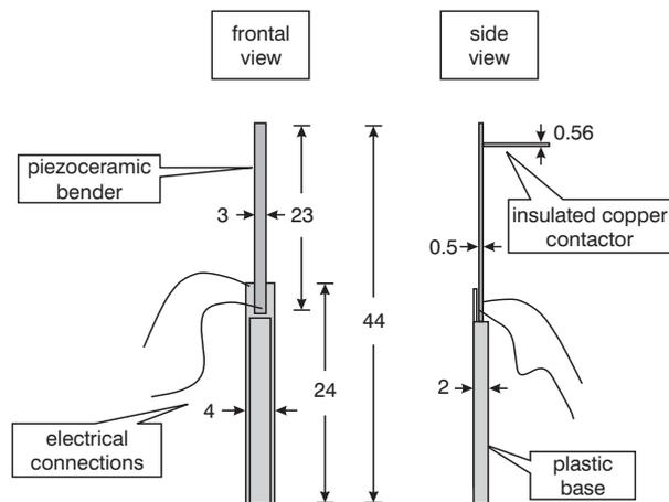
Fig. 3 Detailed schematic diagram of connections and dimensions, in mm, of each piezoelectric vibrator. Frontal and side views are shown
