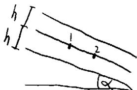
$$\frac{dp}{dx} = \frac{\Delta p}{\Delta x} = \frac{p_1 - p_2}{x_1 - x_2} = \frac{p_1 + \rho g h_1 - p_2 - \rho g h_2}{x_1 - x_2} = \frac{\rho g (h_1 - h_2)}{x_1 - x_2} = -\rho g \sin \alpha$$
