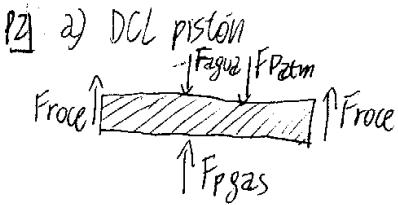
$$\text{vel cte} \Rightarrow \sum F = 0 \Leftrightarrow F_{\text{gases}} + F_{\text{atm}} = F_{\text{gases}} + F_{\text{atm}} \quad (1)$$
