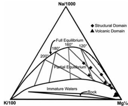
Figure 3. Na-K-Mg diagram (Giggenbach 1988) shows partial equilibrium in most of the cases.
