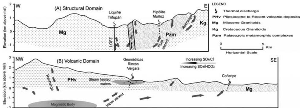
Figure 5. Conceptual model of the geothermal systems for the (a) structural and (b) volcanic domains.
