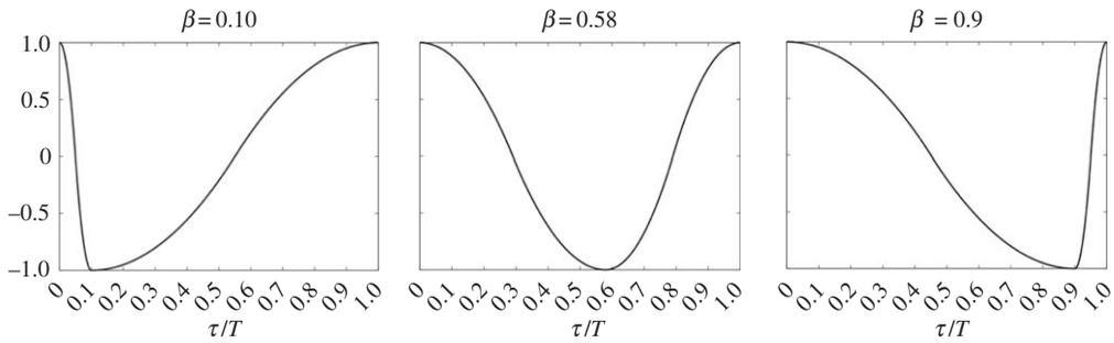
**Figure 2.** The function  $\alpha(\tau; \beta)$  that defines the box-oscillation profile for different values of the asymmetry parameter  $\beta$ . For  $\beta < 1/2$ , the downwards interval takes a shorter time than the upward movement (left) and conversely for  $\beta > 1/2$  (right). For  $\beta = 1/2$ , the function  $\alpha(\tau; \beta)$  resembles  $\cos(2\pi \tau/T)$ .
