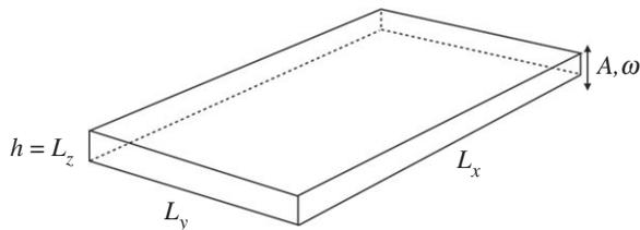
**Figure 1.** Configuration of the Q2D granular system. The box is periodic in the horizontal directions, while it is confined by the top and bottom hard walls. The inner height is  $h$ . Grains are placed inside the box, which is vertically vibrated with amplitude  $A$  and angular frequency  $\omega$ .
