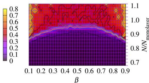
**Figure 8.** Density contrast  $c$  in the  $\beta$ - $N/N_{\text{monolayer}}$  plane for a system with  $L_z = 1.8\sigma$  and  $L_x \times L_y = 90\sigma \times 4.65\sigma$  and vibration parameters  $\tilde{\omega} = \omega/\sqrt{g/\sigma} = 3$  and  $A = 0.29\sigma$ ;  $\zeta = 0.87$ ,  $\Gamma = 2.61$ . The inelasticity and friction grain–grain and grain–wall coefficients are  $r_n = r_t = 0.91$  and  $\mu_d = 0.10$ ,  $\mu_s = 0.17$ . (Online version in colour.)
