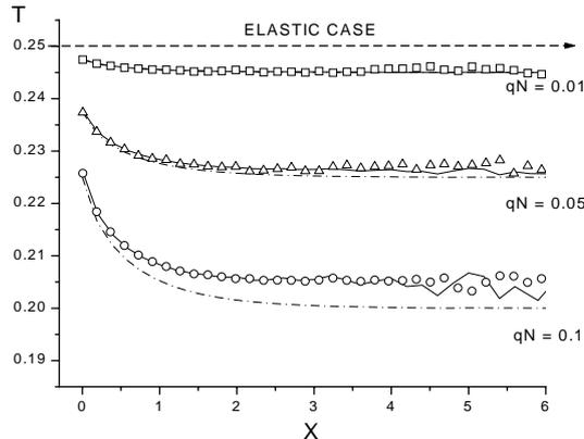
**Fig. 3.** Temperature profiles for  $qN = 0.01$  (squares),  $qN = 0.05$  (triangles) and  $qN = 0.1$  (circles). The solid (dot-dashed) line is the predicted dimensionless temperature up to second (first) order.
