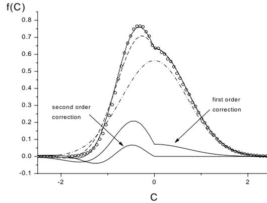
**Fig. 2.** The distribution function normalized to 1 at  $\hat{x} = 0$  evaluated to zeroth (dot-dashed line), first (dashed line) and second order (solid line) are seen in this figure for  $qN = 0.2$  and  $N = 200$ . Circles are the simulational results.
