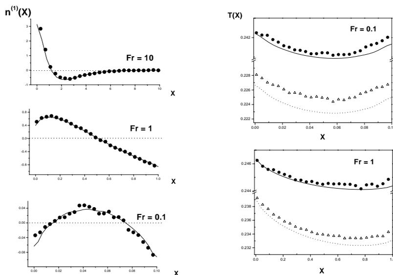
**Fig. 4.** At left, density corrections due to dissipation for different Froude numbers. At right, the temperature profile for two values of the Froude number with  $qN = 0.01$  (dots) and  $qN = 0.03$  (triangles). If  $Fr$  is small enough  $T$  shows a minimum even though the only source of energy is at the bottom. In both cases lines are the theoretical predictions while symbols are the measured data from MD simulations.
