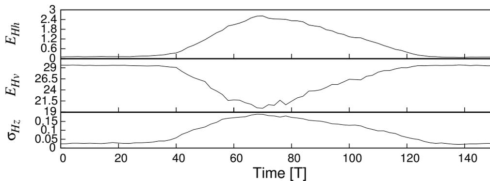
**FIGURE 3.** Evolution of a single energy burst. The average horizontal and vertical energies of the heavy particles  $E_{H_h}$ ,  $E_{H_v}$ , and the standard deviation of the set of heights of particles  $H$ ,  $\sigma_{H_z}$  taken stroboscopically when the box is at its lowest position.
