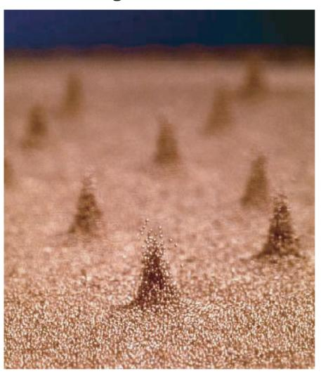
Localized excitations in a vibrating layer of sand (Oscillons)
