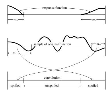
Figure 13.1.3. The wrap-around problem in convolving finite segments of a function. Not only must the response function wrap be viewed as cyclic, but so must the sampled original function. Therefore a portion at each end of the original function is erroneously wrapped around by convolution with the response function.
