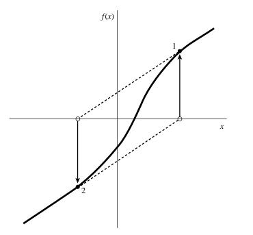
Figure 9.4.3. Unfortunate case where Newton's method enters a nonconvergent cycle. This behavior is often encountered when the function f is obtained, in whole or in part, by table interpolation. With a better initial guess, the method would have succeeded.
