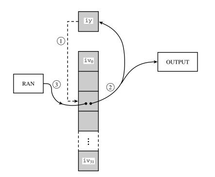
Figure 7.1.1. Shuffling procedure used in ran1 to break up sequential correlations in the Minimal Standard generator. Circled numbers indicate the sequence of events: On each call, the random number in iy is used to choose a random element in the array iv. That element becomes the output random number, and also is the next iy. Its spot in iv is refilled from the Minimal Standard routine.
