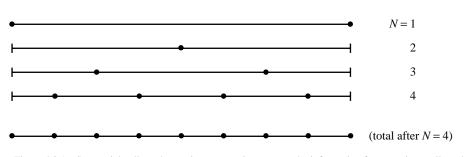
Figure 4.2.1. Sequential calls to the routine trapzd incorporate the information from previous calls and evaluate the integrand only at those new points necessary to refine the grid. The bottom line shows the totality of function evaluations after the fourth call. The routine qsimp, by weighting the intermediate results, transforms the trapzoid rule into Simpson's rule with essentially no additional overhead.
