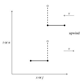
Figure 19.1.4. Representation of upwind differencing schemes. The upper scheme is stable when the advection constant v is negative, as shown; the lower scheme is stable when the advection constant v is positive, also as shown. The Courant condition must, of course, also be satisfied.
