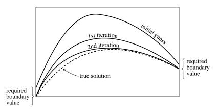
Figure 17.0.2. Relaxation method (schematic). An initial solution is guessed that approximately satisfies the differential equation and boundary conditions. An iterative process adjusts the function to bring it into close agreement with the true solution.
