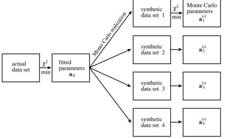
Figure 15.6.2. Monte Carlo simulation of an experiment. The fitted parameters from an actual experiment are used as surrogates for the true parameters. Computer-generated random numbers are used to simulate many synthetic data sets. Each of these is analyzed to obtain its fitted parameters. The distribution of these fitted parameters around the (known) surrogate true parameters is thus studied.
