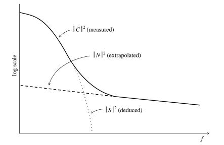
Figure 13.3.1. Optimal (Wiener) filtering. The power spectrum of signal plus noise shows a signal peak added to a noise tail. The tail is extrapolated back into the signal region as a "noise model." Subtracting gives the "signal model." The models need not be accurate for the method to be useful. A simple algebraic combination of the models gives the optimal filter (see text).
