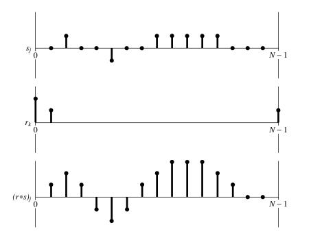
Figure 13.1.2. Convolution of discretely sampled functions. Note how the response function for negative times is wrapped around and stored at the extreme right end of the array  $\eta_c$ .
