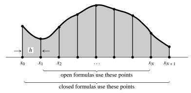
Figure 4.1.1. Quadrature formulas with equally spaced abscissas compute the integral of a function between  $x_0$  and  $x_{N+1}$ . Closed formulas evaluate the function on the boundary points, while open formulas refrain from doing so (useful if the evaluation algorithm breaks down on the boundary points).
