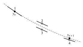
Figure 16.1.3. Fourth-order Runge-Kutta method. In each step the derivative is evaluated four times: once at the initial point, twice at trial midpoints, and once at a trial endpoint. From these derivatives the final function value (shown as a filled dot) is calculated. (See text for details.)
