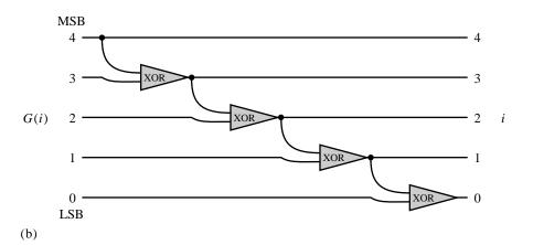
Figure 20.2.1. Single-bit operations for calculating the Gray code G(i) from i (a), or the inverse (b). LSB and MSB indicate the least and most significant bits, respectively. XOR denotes exclusive-or.
