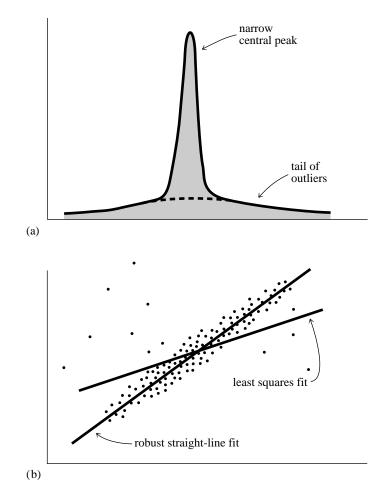
Figure 15.7.1. Examples where robust statistical methods are desirable: (a) A one-dimensional distribution with a tail of outliers; statistical fluctuations in these outliers can prevent accurate determination of the position of the central peak. (b) A distribution in two dimensions fitted to a straight line; non-robust techniques such as least-squares fitting can have undesired sensitivity to outlying points.
