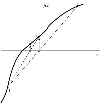
Figure 9.2.2. False position method. Interpolation lines (dashed) are drawn through the most recent points *that bracket the root*. In this example, point 1 thus remains "active" for many steps. False position converges less rapidly than the secant method, but it is more certain.
