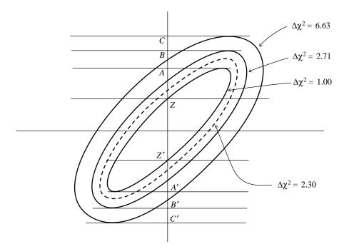
Figure 15.6.4. Confidence region ellipses corresponding to values of chi-square larger than the fitted minimum. The solid curves, with  $\Delta\chi^2 = 1.00, 2.71, 6.63$  project onto one-dimensional intervals AA', BB', CC'. These intervals — not the ellipses themselves — contain 68.3%, 90%, and 99% of normally distributed data. The ellipse that contains 68.3% of normally distributed data is shown dashed, and has  $\Delta\chi^2 = 2.30$ . For additional numerical values, see accompanying table.
