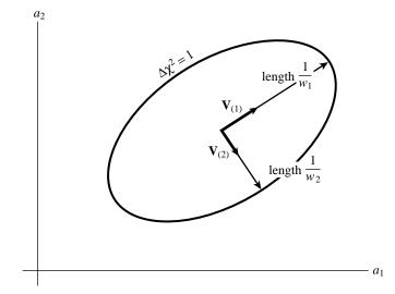
Figure 15.6.5. Relation of the confidence region ellipse  $\Delta \chi^2 = 1$  to quantities computed by singular value decomposition. The vectors  $\mathbf{V}_{(i)}$  are unit vectors along the principal axes of the confidence region. The semi-axes have lengths equal to the reciprocal of the singular values  $u_i$ . If the axes are all scaled by some constant factor  $\alpha$ ,  $\Delta \chi^2$  is scaled by the factor  $\alpha^2$ .
