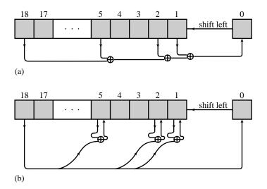
Figure 7.4.1. Two related methods for obtaining random bits from a shift register and a primitive polynomial modulo 2. (a) The contents of selected taps are combined by exclusive-or (addition modulo 2), and the result is shifted in from the right. This method is easiest to implement in hardware. (b) Selected bits are modified by exclusive-or with the leftmost bit, which is then shifted in from the right. This method is easiest to implement in software.
