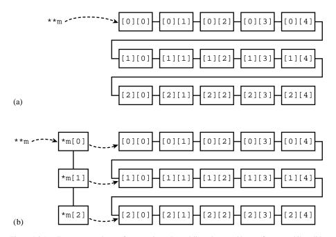
Figure 1.2.1. Two storage schemes for a matrix m. Dotted lines denote address reference, while solid lines connect sequential memory locations. (a) Pointer to a fixed size two-dimensional array. (b) Pointer to an array of pointers to rows; this is the scheme adopted in this book.
