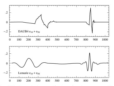
Figure 13.10.2. More wavelets, here generated from the sum of two unit vectors,  $\mathbf{e}_{10} + \mathbf{e}_{58}$ , which are in different hierarchical levels of scale, and also at different spatial positions. DAUB4 wavelets (a) are defined by a filter in coordinate space (equation 13.10.5), while Lemarie wavelets (b) are defined by a filter most easily written in Fourier space (equation 13.10.14).
