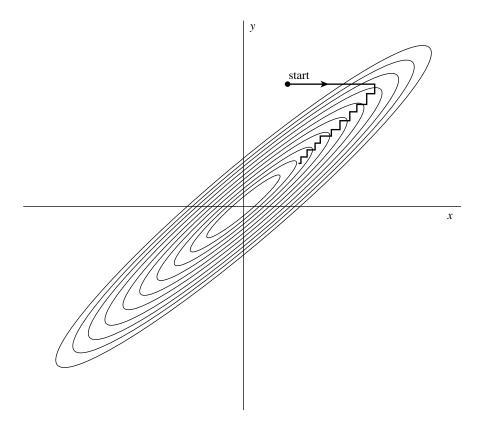
Figure 10.5.1. Successive minimizations along coordinate directions in a long, narrow "valley" (shown as contour lines). Unless the valley is optimally oriented, this method is extremely inefficient, taking many tiny steps to get to the minimum, crossing and re-crossing the principal axis.
