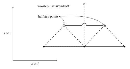
Figure 19.1.7. Representation of the two-step Lax-Wendroff differencing scheme. Two halfstep points  $(\otimes)$  are calculated by the Lax method. These, plus one of the original points, produce the new point via staggered leapfrog. Halfstep points are used only temporarily and do not require storage allocation on the grid. This scheme is second-order accurate in both space and time.
