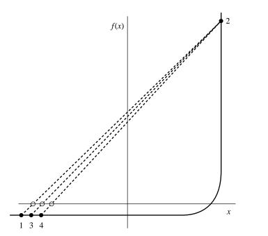
Figure 9.2.3. Example where both the secant and false position methods will take many iterations to arrive at the true root. This function would be difficult for many other root-finding methods.
