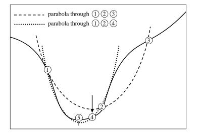
Figure 10.2.1. Convergence to a minimum by inverse parabolic interpolation. A parabola (dashed line) is drawn through the three original points 1,2,3 on the given function (solid line). The function is evaluated at the parabola's minimum, 4, which replaces point 3. A new parabola (dotted line) is drawn through points 1,4,2. The minimum of this parabola is at 5, which is close to the minimum of the function.
