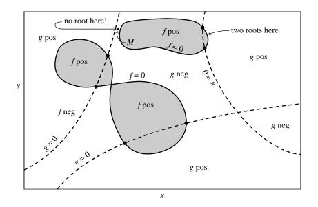
Figure 9.6.1. Solution of two nonlinear equations in two unknowns. Solid curves refer to f(x, y), dashed curves to g(x, y). Each equation divides the (x, y) plane into positive and negative regions, bounded by zero curves. The desired solutions are the intersections of these unrelated zero curves. The number of solutions is *a priori* unknown.
