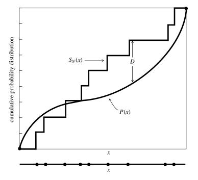
Figure 14.3.1. Kolmogorov-Smirnov statistic D. A measured distribution of values in x (shown as N dots on the lower abscissa) is to be compared with a theoretical distribution whose cumulative probability distribution is plotted as P(x). A step-function cumulative probability distribution  $S_N(x)$  is constructed, one that rises an equal amount at each measured point. D is the greatest distance between the two cumulative distributions.
