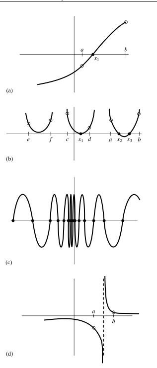
Figure 9.1.1. Some situations encountered while root finding: (a) shows an isolated root  $x_1$  bracketed by two points a and b at which the function has opposite signs; (b) illustrates that there is not necessarily a sign change in the function near a double root (in fact, there is not necessarily a root!); (c) is a pathological function with many roots; in (d) the function has opposite signs at points a and b, but the points bracket a singularity, not a root.
