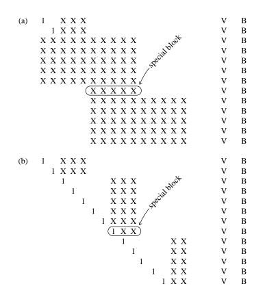
Figure 17.6.1. FDE matrix structure with an internal boundary condition. The internal condition introduces a special block. (a) Original form, compare with Figure 17.3.1; (b) final form, compare with Figure 17.3.2.
