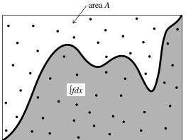
Figure 7.6.1. Monte Carlo integration. Random points are chosen within the area A. The integral of the function f is estimated as the area of A multiplied by the fraction of random points that fall below the curve f. Refinements on this procedure can improve the accuracy of the method; see text.
