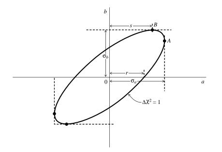
Figure 15.3.1. Standard errors for the parameters a and b. The point B can be found by varying the slope b while simultaneously minimizing the intercept a. This gives the standard error  $\sigma_b$ , and also the value s. The standard error  $\sigma_a$  can then be found by the geometric relation  $\sigma_a^2 = s^2 + r^2$ .
