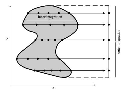
Figure 4.6.1. Function evaluations for a two-dimensional integral over an irregular region, shown schematically. The outer integration routine, in y, requests values of the inner, x, integral at locations along the y axis of its own choosing. The inner integration routine then evaluates the function at x locations suitable to *it*. This is more accurate in general than, e.g., evaluating the function on a Cartesian mesh of points.
