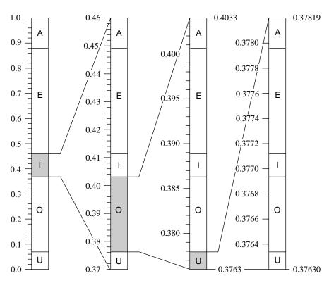
Figure 20.5.1. Arithmetic coding of the message "IOU..." in the fictitious language Vowellish. Successive characters give successively finer subdivisions of the initial interval between 0 and 1. The final value can be output as the digits of a fraction in any desired radix. Note how the subinterval allocated to a character is proportional to its probability of occurrence.
