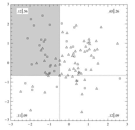
Figure 14.7.1. Two-dimensional distributions of 65 triangles and 35 squares. The two-dimensional K–S test finds that point one of whose quadrants (shown by dotted lines) maximizes the difference between fraction of triangles and fraction of squares. Then, equation (14.7.1) indicates whether the difference is statistically significant, i.e., whether the triangles and squares must have different underlying distributions.
