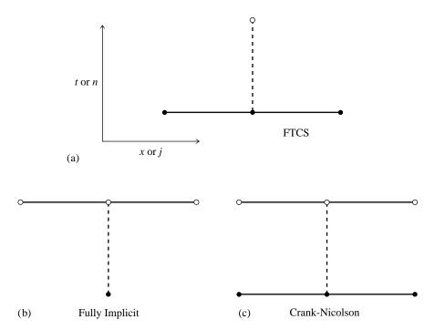
Three differencing schemes for diffusive problems (shown as in Figure 19.1.2). (a) Figure 19.2.1. Forward Time Center Space is first-order accurate, but stable only for sufficiently small timesteps. (b) Fully Implicit is stable for arbitrarily large timesteps, but is still only first-order accurate. (c) Crank-Nicolson is second-order accurate, and is usually stable for large timesteps.
