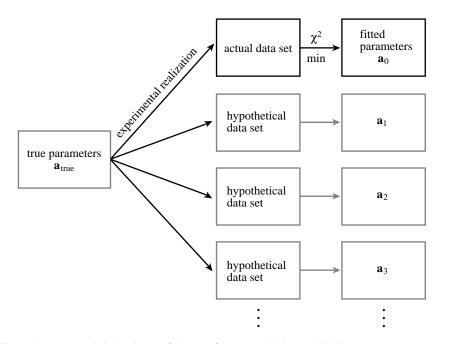
Figure 15.6.1. A statistical universe of data sets from an underlying model. True parameters  $\mathbf{a}_{true}$  are realized in a data set, from which fitted (observed) parameters  $\mathbf{a}_0$  are obtained. If the experiment were repeated many times, new data sets and new values of the fitted parameters would be obtained.
