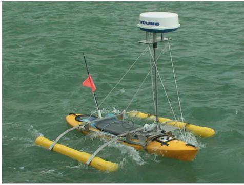
Fig. 6. The Autonomous Surface Craft (ASC) adapted kayak.
