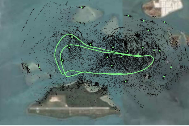
Fig. 7. Overview of the test site showing the GPS trajectory (green line) and AIS coordinates (green dots) of the point feature map. The point feature measurement history is also provided (black dots).
