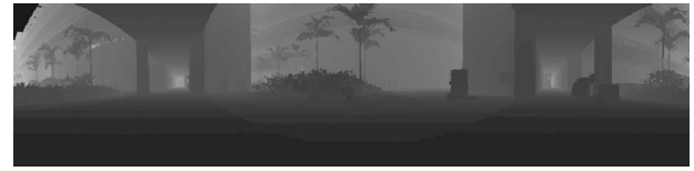
Figure 23. The corresponding range image of the scan in Figure 22. Darker pixels are closer to the sensor.
