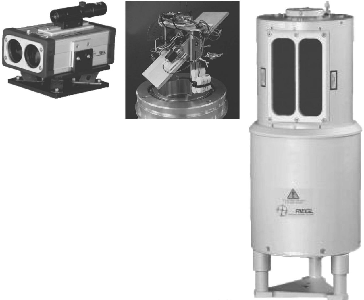
Figure 1. (a) 1D Riegl LADAR LD90-3300EHS-FLP model, (b) in-house developed 3D scanning mechanism, and (c) 3D Riegl LADAR LMS-Z210i. The 3D mechanism in (b) and the 3D LADAR in (c) allow continuous rotation of the scanning mirror about the vertical axis and simultaneous control of the mirror's elevation about a horizontal axis.
