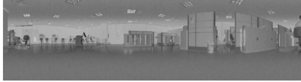
Figure 2. Received signal amplitude image recorded in a laboratory environment. Each pixel value is proportional to the received signal amplitude. The small circle (labelled "A") shows a zero-signal amplitude point.
