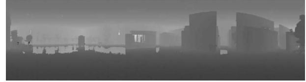
Figure 3. The corresponding range image of the scan in Figure 2. Each pixel value is proportional to the estimated range. Darker pixels show closer objects.
