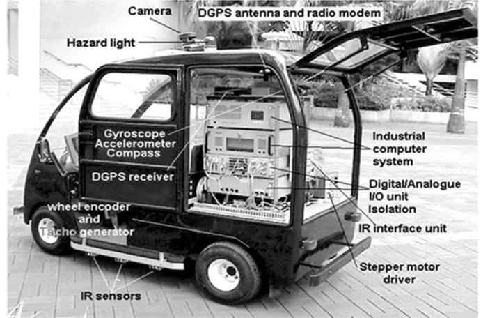
Fig. 11. Mobile robot used in SLAM experiments.
