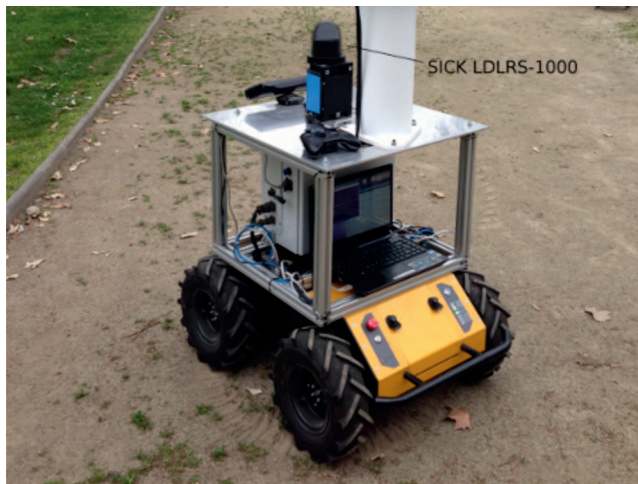
Fig. 7. Vehicle platform and scanning laser range finder used in generating Parque O'Higgins data set.
