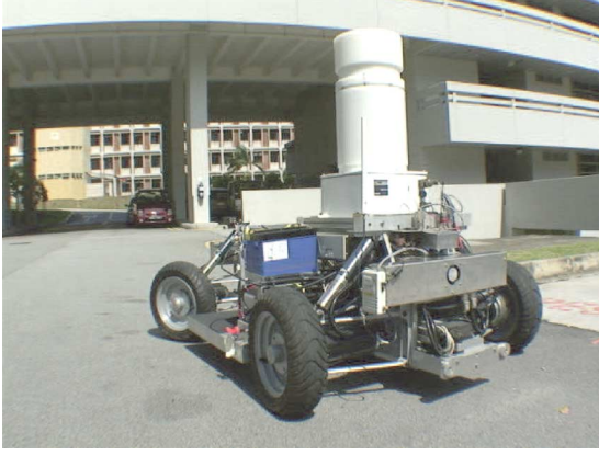
Fig. 1. Photograph of the MMW radar used in the experiments. The antenna (located at the bottom of the unit) and swash plate (located in the cylindrical central section) are housed in an almost opaque perspex housing.
