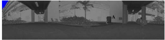
Fig. 14. An intensity image of an semi-outdoor environment from the 1D-sensor based 3D LADAR. 'A' in the figure denotes a container.
