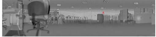
Fig. 18. Received signal amplitude image recorded in the same laboratory environment in figure 2 by the 3D LADAR in figure 1(c). 'A' denotes a container.
