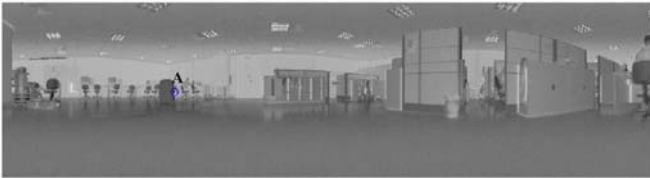
Fig. 2. Received signal amplitude image recorded in a laboratory environment. Each pixel value is proportional to the received signal amplitude. The small circle (labelled with “A”) shows a zero-signal amplitude point.
