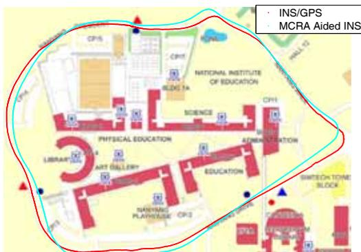
Fig. 6. The red curve is the path from INS/GPS as the ground truth. The cyan one is the MCRA aided INS path.
