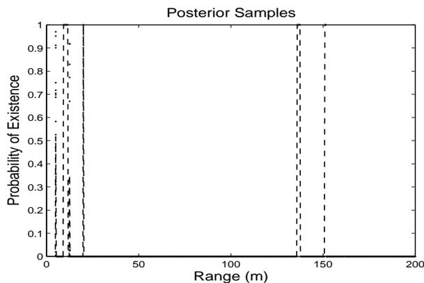
Fig. 8. The posterior occupancy samples, after five filter iterations, with the dashed line again representing the mean existence in each bin.
