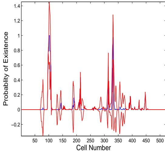
Fig. 15. A cross section through the map showing the estimate occupancy with 2 sigma bounds. For illustration purposes the bounds are not cropped at the variable bounded limits of 0 and 1.
