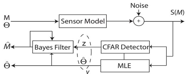
Fig. 3. A block diagram of the proposed algorithm. The aim is to estimate the posterior on the occupancy vector,  $M$ . This however requires estimates of the measurement likelihoods  $\hat{\Theta}$ .  $y$  represents the measurements used in the Bayes filter.
