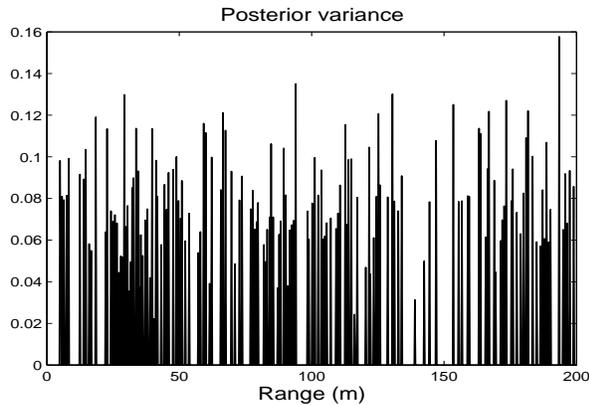
Fig. 7. Variance of the posterior occupancy samples, in each range bin  $k$ , after a single filter iteration.
