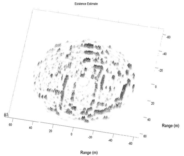
Fig. 13. A plot of the mean existence value on the map. The model considered missed detections of objects with low radar cross section unlike that of the log odds model.
