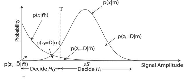
Fig. 1. A graphical representation of the received signal classification problem.  $T$  represents the decision threshold,  $\mu$  is the mean noise power and  $S$  is the mean target signal-to-noise ratio. The hypothesis decisions are  $H_0$ : Target absent, and  $H_1$ : Target present. The measurement likelihoods required to calculate the posterior probability of occupancy are also indicated.
