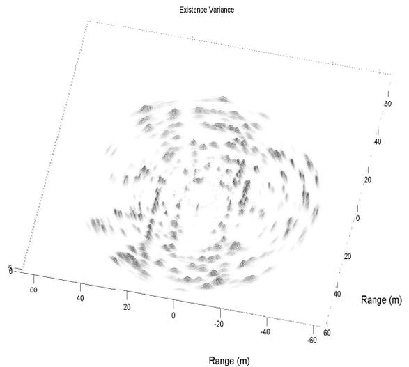
Fig. 14. A plot of the variance of the occupancy estimates. This allows us to statistically quantify the occupancy estimates on the map which is not considered in previous methods.
