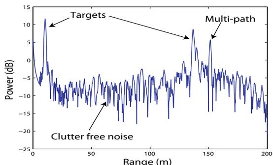
Fig. 2. A sample spectrum, from a frequency modulated continuous wave radar, containing  $K$  (assumed independent) signal measurements,  $s_k$ , at  $K$  range bins for a single sensor bearing angle.
