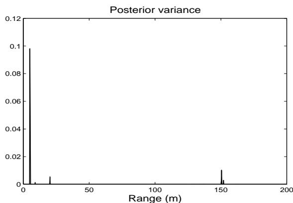
Fig. 9. Variance of the posterior occupancy samples, after five filter iterations. The filter is most certain of landmark existence at 135m as there is low variance on a high occupancy estimate.
