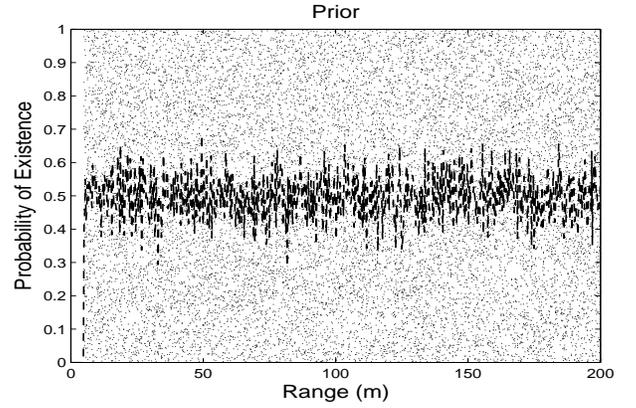
Fig. 4. The uniform *a priori* occupancy samples at each range bin with the mean (dashed) plotted
