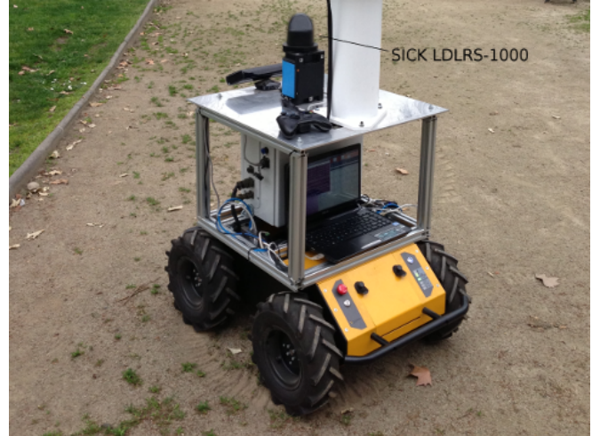
Fig. 1: The robotic platform and scanning laser range finder used in generating the experimental dataset.
